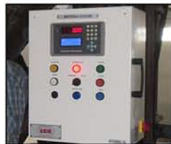
Batch Weighing System
